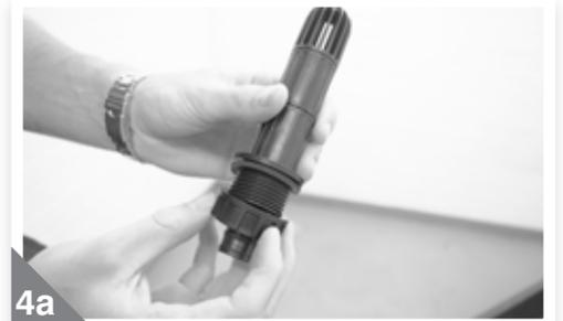
Remove the nut from the overflow fitting.
